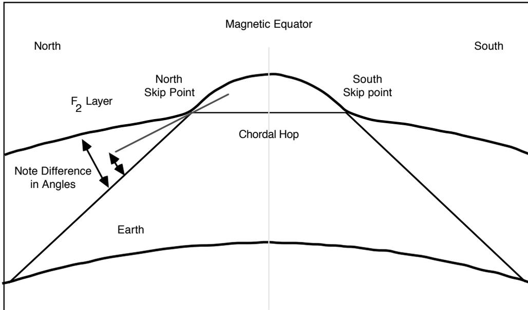
*Figure 5.* A diagram of a transequatorial chordal hop off the tilted north and south skip points. These points lie about 20° north and south of the Earth's magnetic equator and can be major contributors to daytime transequatorial six-meter propagation from mid latitudes and clearly cause nighttime TEP in the tropics.
