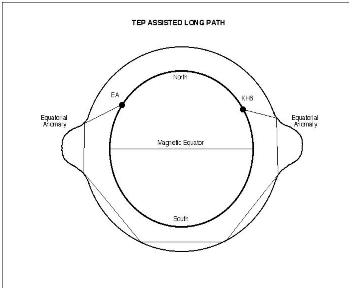
Figure 7. TEP can provide the launching points for shallow attack angle grazing hops that cover long distances, with higher than normal MUF's and low absorption. At such times, long-path can be a superior mode of propagation
