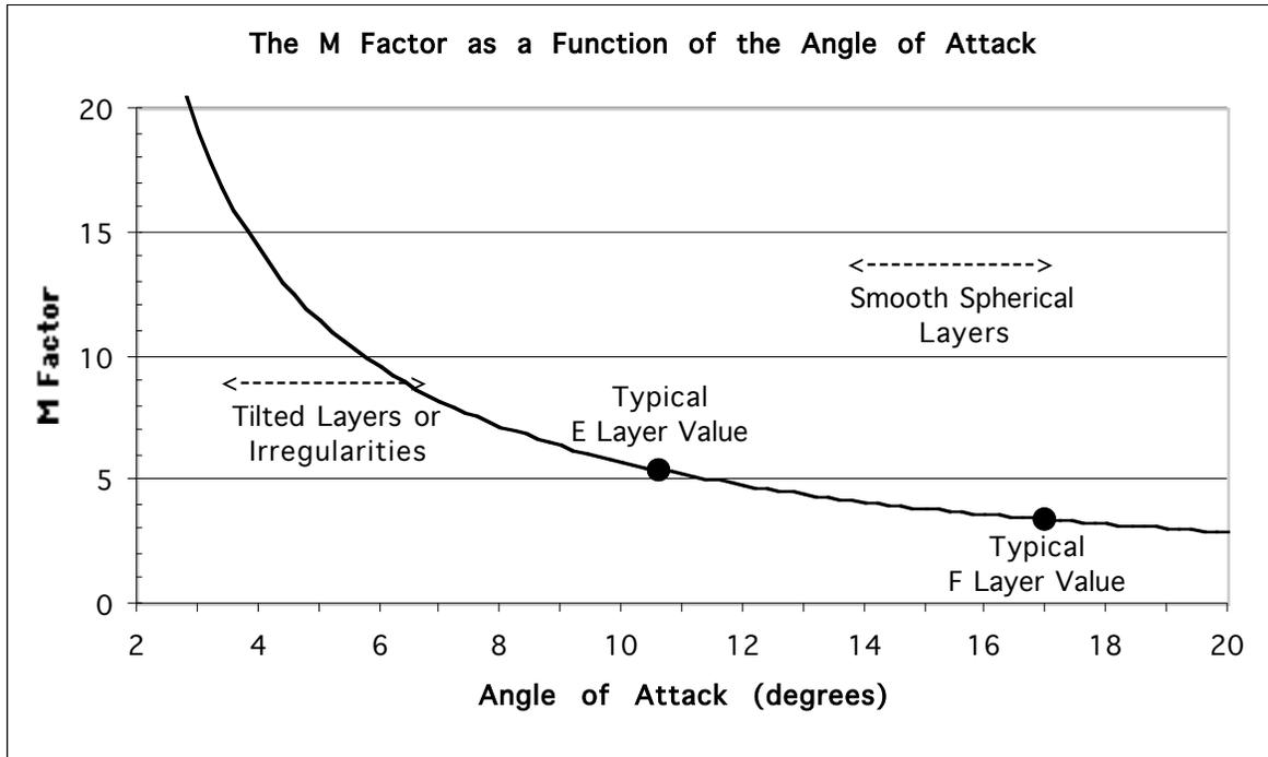
Figure 2.  $M$  varies with angle of attack. A smooth spherical ionosphere gives angles between 10 and 20 degrees. Lower layers lead to smaller angles, larger  $M$ 's, and higher MUF's, for same ionization. For VHF, tilted layers or other irregularities can produce angles below 10 degrees and provide very exciting results. In the extreme, TEP on 222 MHz and higher can result
